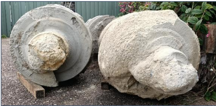
Figure 17: Pile base formed in silt (left) and in sand (right)
