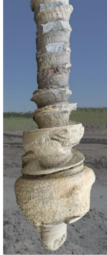
Figure 18: Pile shaft after removal of helical thread
